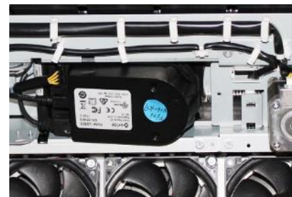
The X-Rite® Inline Spectrophotometer automates the collection of XRG data for calibration and profiling.
